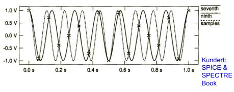
**Figure 5.9:** An example of aliasing. The seventh and ninth harmonics are sampled at a rate of 16 per period of the fundamental. Notice that the values of both waveforms are identical at the sample points.
