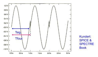
**Figure 5.7:** The 1 second periodic extension of a 1.05 Hz sinewave. A large difference between the period of the sinewave and the period of the extension was used to make the discontinuity visible in a time-domain waveform. The spectrum of a sinewave with a much smaller difference is shown in Figure 5.8 on the following page.
