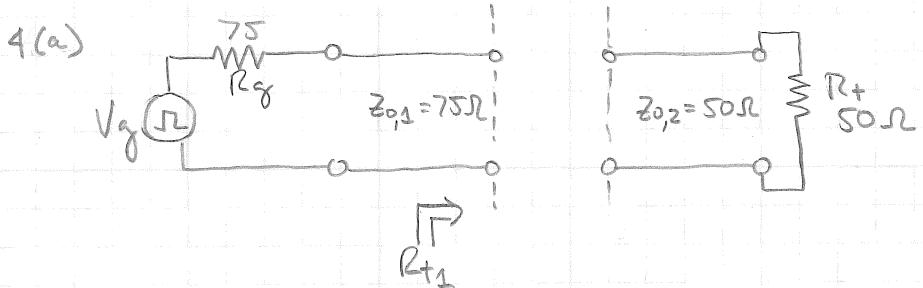
In this case, a wavefront from the left encountering the boundary  $R_{+1}$  should see an impedance of  $75\Omega$ . Since the right-hand side of the boundary is at a lower impedance, the only connection for the resistor that will present a higher impedance to the wavefront will be a series one that when added to  $z_{0,2}$  equals  $75\Omega$ . This would be a  $25\Omega$  series resistor.
