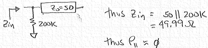
No reflections will occur at points B+C. The full size incident wave will correctly be received at points B+C, and no reflections will be generated, thus no termination is required.
