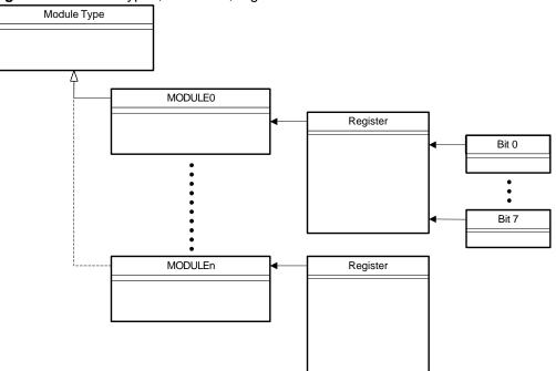
Figure 2-1. Module types, instances, registers and bits.
